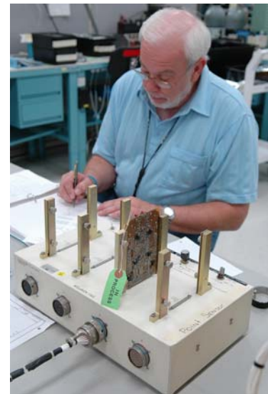
LLOYD PIERCE, a NASA test engineer, checks electronic components related to the faulty sensor readings in the liquid hydrogen tank low-level fuel cut-off sensor. The sensor failed a routine prelaunch check during the launch attempt July 13.
