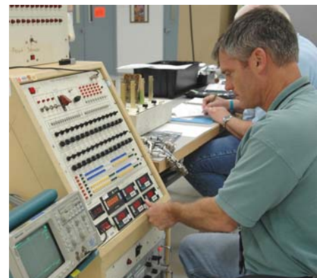
GARY KING helps test electronic components related to the faulty sensor readings in the liquid hydrogen tank low-level fuel cut-off sensor.
