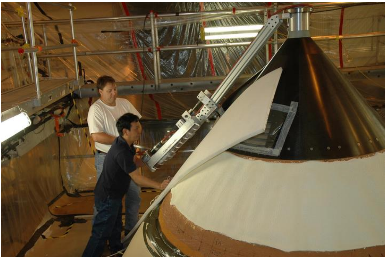
In NASA Kennedy Space Center's Vehicle Assembly Building, one technician adjusts the sander while another observes as they work on repairing the hail damage to Atlantis' nose cone.
