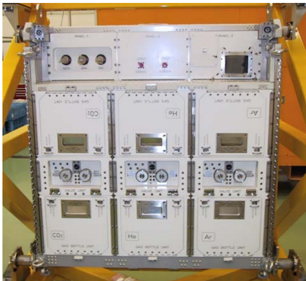
Common Gas Supply Equipment
