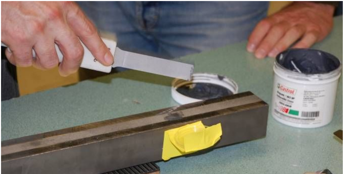
The SARJ scraper tool in combination with a lubricant (602 Braycote EF) will be used as a cleaning tool on the outer canted surface.
