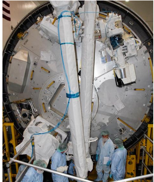
Launch configuration of the JEMRMS
