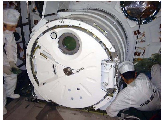
JEM airlock as seen from the PM interior. Note that the inner hatch is equipped with a window, a pressure gauge and operating handle.
