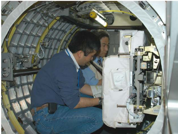
JAXA astronaut Koichi Wakata reviewing procedures for removal of the JEM airlock forward launch locks
