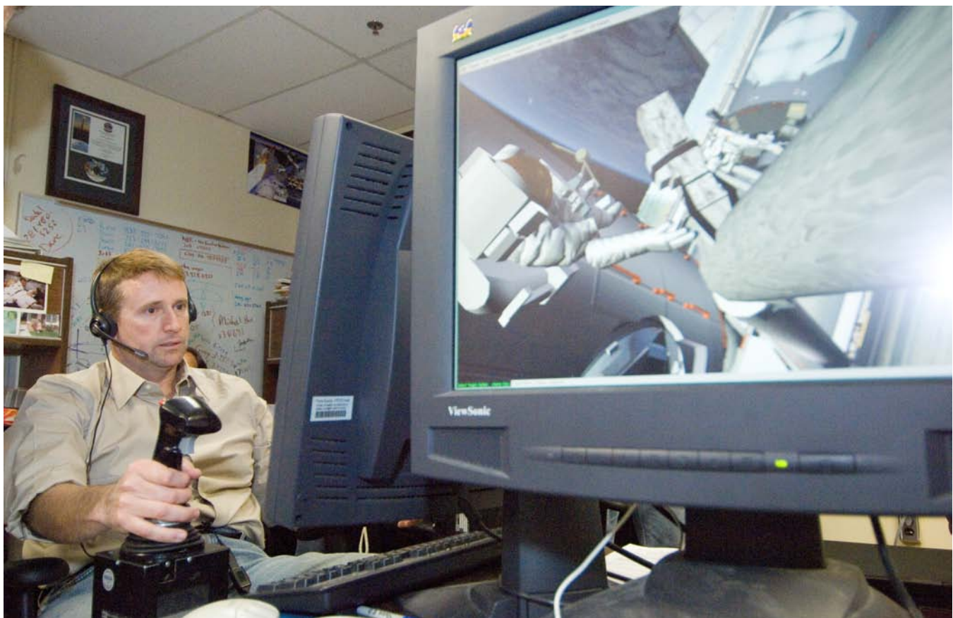
Astronaut Ken Ham, STS-124 pilot, uses the virtual reality lab at JSC to train for some of his duties aboard the space shuttle and space station. This type of computer interface, paired with virtual reality training hardware and software, helps to prepare the entire team for dealing with space station elements.
